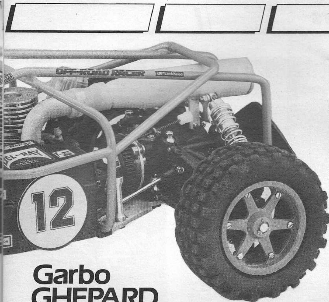
Above: the 'Ghepard' has a very large suspension movement, 3in. on each wheel whilst still keep the other three on the ground.
